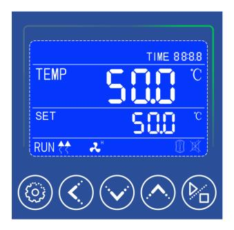
1. The button permits the working parameters setting and to enter/escape from the programs (PRO version only).
